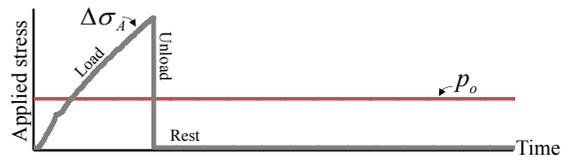
Figure 2. Scheme of applied stress history, consisting of a timewise constant confinement level and a sequence of load-unload-rest in axial compression.
