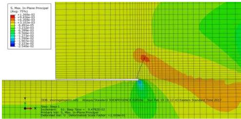
Figure 9. Plot of maximum stresses (+ is tension) and crack propagation for  $\tau/\sigma_n > 1$
