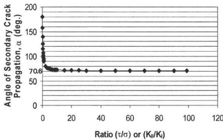
Figure 7. Angle of secondary crack propagation for any value of the ratio ( $\tau/\sigma$ ) or ( $K_{II}/K_I$ )
