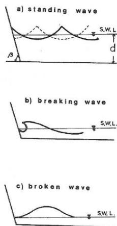
Figure 4. Different wave types acting at the toe of coastal slopes.
