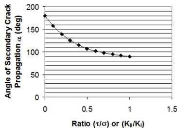
Figure 8. Angle of secondary crack propagation for any value of the ratio ( $\tau/\sigma$ ) or ( $K_{II}/K_I$ ) between 0 and 1.
