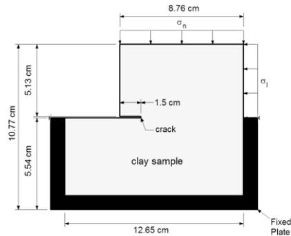
Figure 3. A clay slope with an open crack at its toe for testing in the PSDSA.
