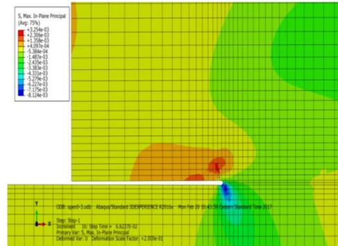
Figure 11. Plot of maximum stresses (+ is tension) and crack propagation for  $\tau/\sigma_n < 1$
