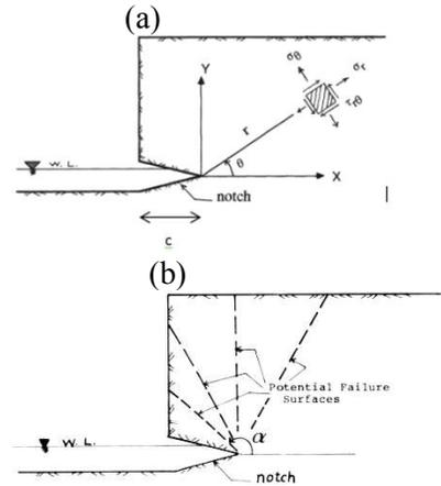
Figure 6. (a) Stresses in the intact material near the tip of a notch; (b) Angles of secondary cracks
