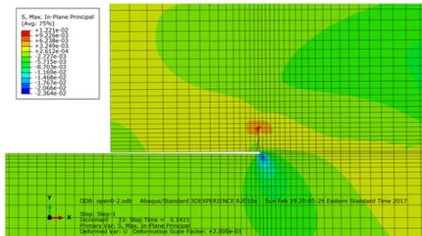
Figure 10. Plot of maximum stresses (+ is tension) and crack propagation for  $\tau/\sigma_n = 1$
