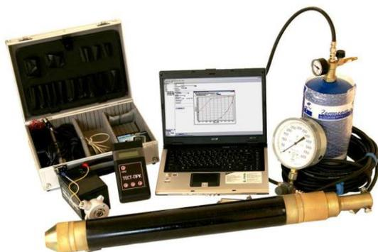
Figure 6. Automatic pressuremeter device for in-situ tests in bore holes
