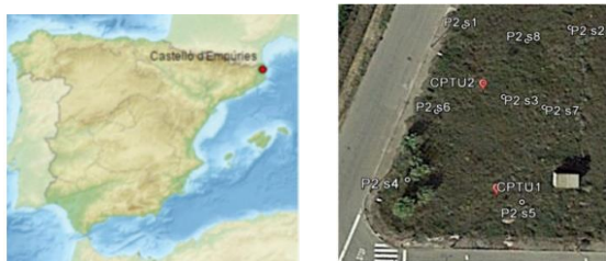
Figure 2. Test site location (dot) and implantation of piezocone tests (CPTU i ) and Panda tests (P2Si)
