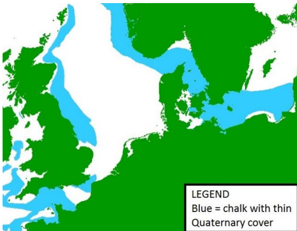
Figure 1. Chalk areas of North Sea and Baltic Sea, water depths of < 50 m (after Ziegler, 1990)
