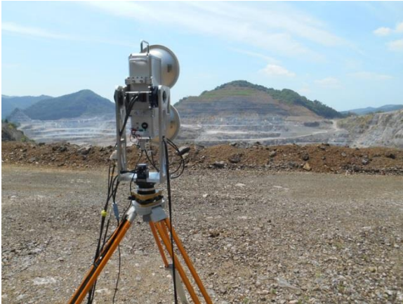
Figure 1. Appearance of ground-based millimeter wave radar.
