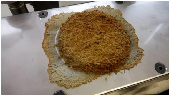
Figure 3. State of the lower part of soil sample post-test and after container removal
