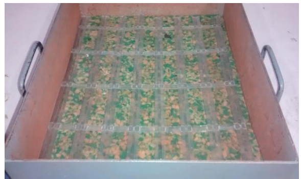
Figure 6. View of the geogrid placed on top of the sponge during specimen preparation
