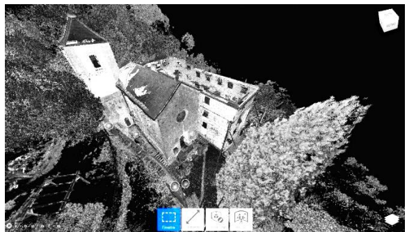
Figure 2: 3D laser scanner survey
