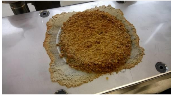
Figure 3. State of the lower part of soil sample post-test and after container removal
