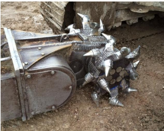
Figure 4. Mass mixing tool (courtesy of Ground Developments Ltd)
