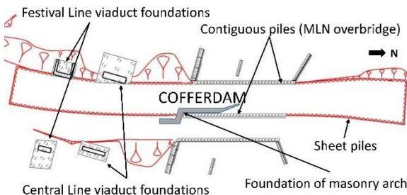
Figure 1. Cofferdam and site constraints
