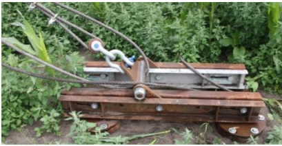
Figure 9. Anchoring with 4 Spinnankers (Type XII / 6,0 / 15)
