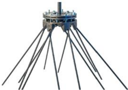
Figure 1. Spinnanker XII / 2.0 / 15 (this Spinnanker comprises 12 threaded bars with a length of 2.0 m and a nominal diameter of 15 mm) - (Product prospect Spinnanker)
