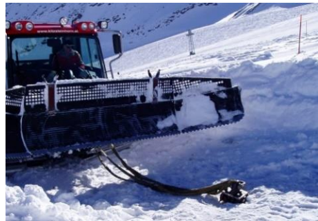
Figure 3. Horizontal pull out test of a Spinnanker VI / 3.0 / 15 on a glacier in Zell am See, Austria (2009)
