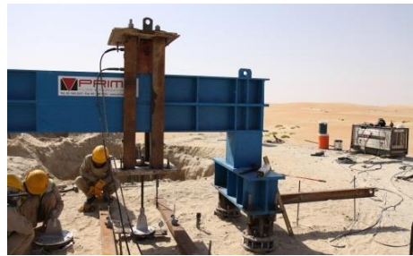
Figure 2. In situ load test for a mobile phone tower in Abu Dhabi, UAE (2014)
