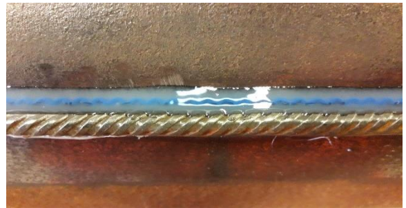
Figure 2. Installation of strain DFOS on the steel piles.
