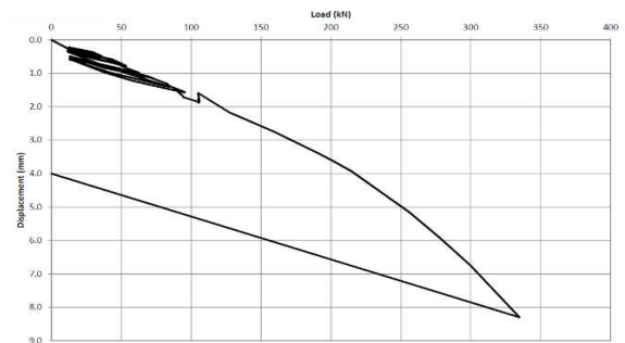
Figure 5: Load displacement graph for the test pile at tower location C26
