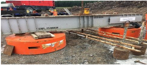
Figure 3: Pile test beam set-up
