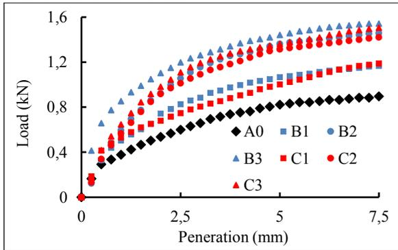
Figure 4. Load penetration curves for unreinforced and FRS samples
