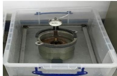
Figure 2. CBR sample in soaked condition
