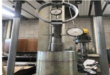
Figure 3. CBR penetration apparatus
