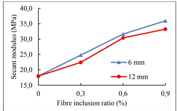
Figure 7. Variation of secant modulus with fibre inclusion ratio at different lengths
