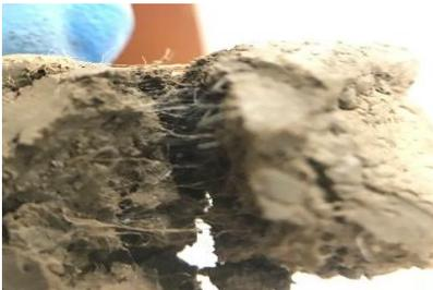
Figure 1. Soil-Fibre composite after mixing
