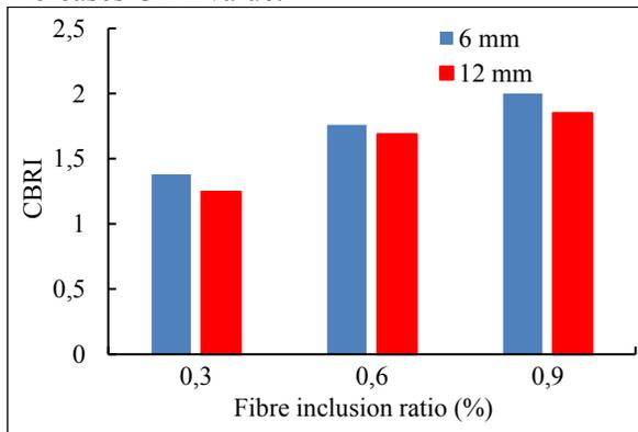
Figure 6. Variation of CBR Index with fibre inclusion ratio at different lengths
