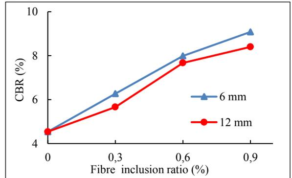
Figure 5. Variation of CBR value with fibre inclusion ratio at different fibre lengths
