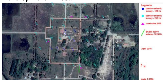
Figure 4. Geotechnical and geophysical prospection implemented in Lumbini in April 2016.
