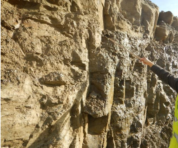
Figure 5. Molassic rock with principal joint layers and joint surfaces
