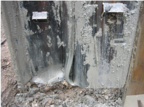
Figure 3 Damaged toe, from Guillemet (2013).
