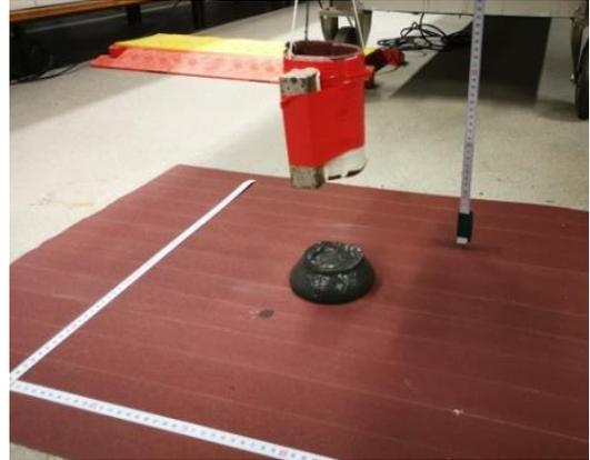
Figure 5: Slump test execution.
