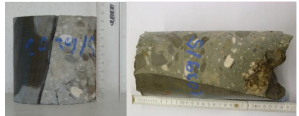
Figure 2. Example for a sample of quality class D (unsuitable)
