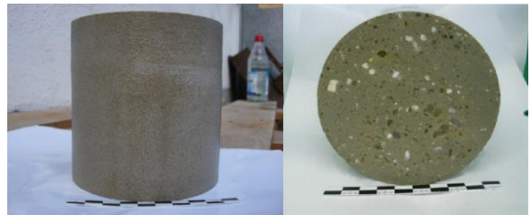
Figure 1. Example for a sample of quality class A (suitable)
