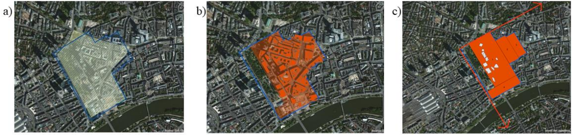
Figure 2. a) the study area; b) low-rise buildings (in orange) whose loads are spread over the test area (framed in blue) with the exclusion of the park; c) the area where the pre-consolidation load was applied (in orange), the footprint area of high-rise buildings (in gray) and the reference axis (in red).
