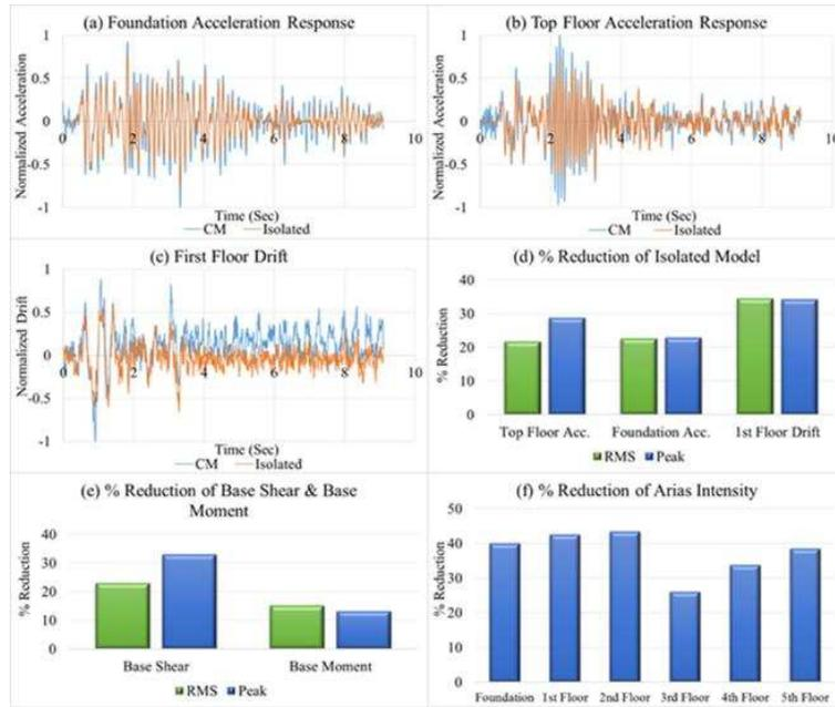
Figure 4. (a) Foundation, (b) Top Floor Horizontal Acceleration Response, (c) First Floor Drift, (d) % Reduction of Isolated Model, (e) % Reduction of Base Shear & Base Moment and (f) % Reduction of Arias Intensity of Isolated Model Comparing CM under Kocaeli Earthquake.
