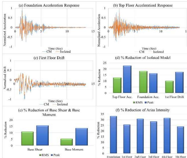
Figure 6. (a) Foundation, (b) Top Floor Horizontal Acceleration Response, (c) First Floor Drift, (d) % Reduction of Isolated Model, (e) % Reduction of Base Shear & Base Moment and (f) % Reduction of Arias Intensity of Isolated Model Comparing CM under Kobe Earthquake.
