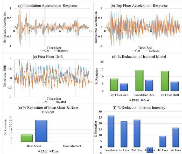
Figure 5. (a) Foundation, (b) Top Floor Horizontal Acceleration Response, (c) First Floor Drift, (d) % Reduction of Isolated Model, (e) % Reduction of Base Shear & Base Moment and (f) % Reduction of Arias Intensity of Isolated Model Comparing CM under El Centro Earthquake.
