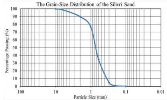
Figure 1. Grain-size distribution of the Silivri Sand.
