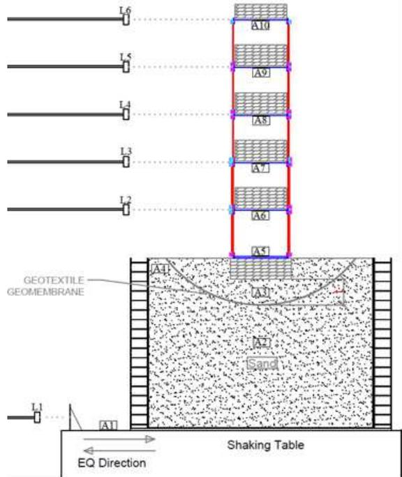
Figure 2. Sketch of Proposed GSI System Experiment Setup with Five-Story Building Model.
