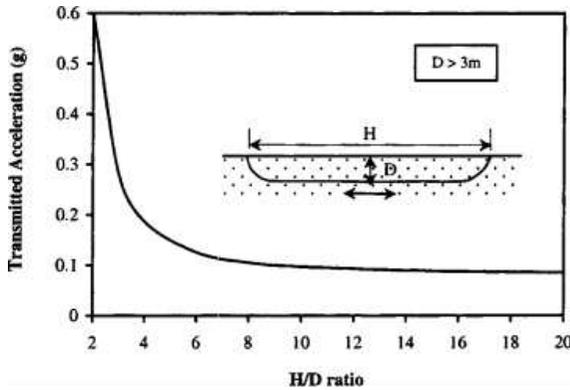
Figure 2. Transmitted Acceleration as a Function of H/D Ratio (Yegian and Catan 2004).
