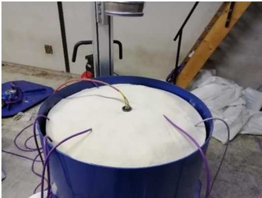
Figure 8: Prepared sample for the experience before the placement of the lid
