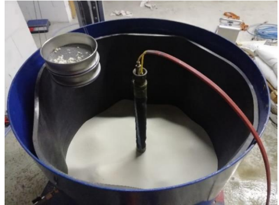
Figure 14: Pluviation of the sand sample in the calibration chamber
