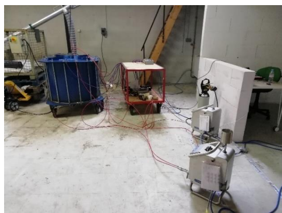
Figure 15: System of pressurization of the probe and the airbags in the same time
