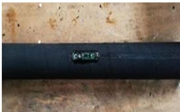
Figure 4: Sensor integrated in the flexible rubber
