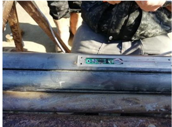
Figure 2: Electronic board inserted in the slotted tube
