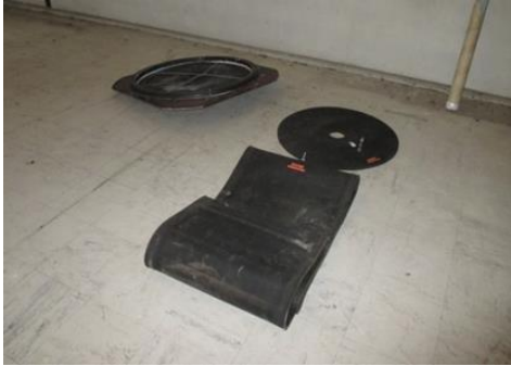
Figure 7: Airbags for the simulation of the lateral and vertical forces
