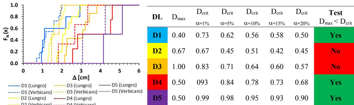
Figure 4. Results of two-sample K-S goodness-of-fit test used to compare, for each considered damage severity level (D1,...,D5) the two samples of masonry building surveyed in Lungro and Verbicaro study areas.
