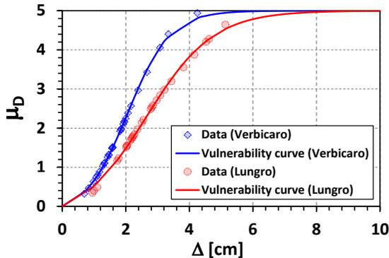
Figure 5. Empirical vulnerability curves for masonry buildings in Lungro and Verbicaro areas.
