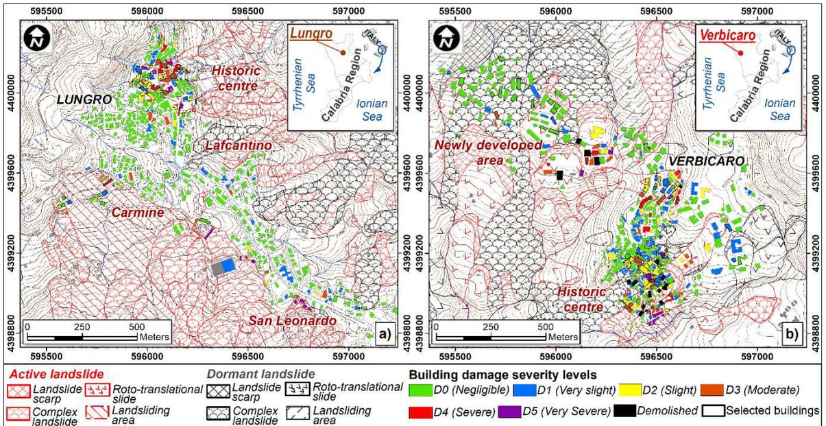
Figure 1. The study areas of a) Lungro and b) Verbicaro: inventory maps of the slow-moving landslides classified based on their state of activity and surveyed buildings distinguished according to the recorded damage severity levels.
