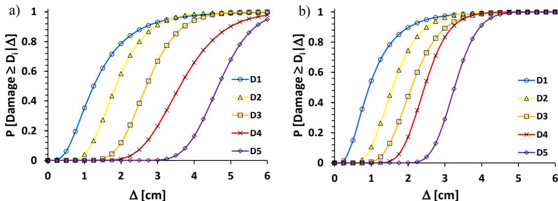
Figure 3. Empirical fragility curves for masonry buildings in a) Lungro and b) Verbicaro study areas.
