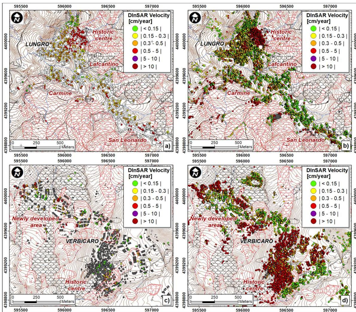
Figure 2. DInSAR velocity distribution derived from SAR images acquired on ascending orbit by ENVISAT (period 2003–2010) radar sensor over the Lungro (a) and Verbicaro study areas (c) and acquired on ascending orbit by COSMO-SkyMed (period 2012–2014) radar sensor over the Lungro (b) and Verbicaro study areas (d).
