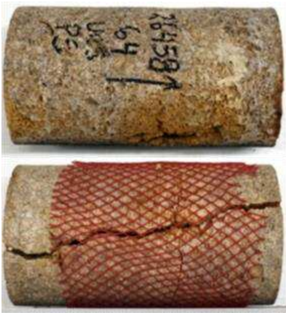
Figure 4. UCS sample that has an existing fracture (top). The fracture is activated during the test (bottom) and samples shows a low UCS-value.
