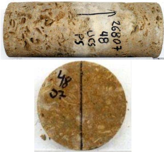
Figure 6. Both samples from the same material. UCS sample (top) is porous but BTS sample (bottom) is not porous.
