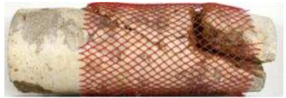
Figure 5. UCS sample with mainly local fracturing (at top of the sample).
