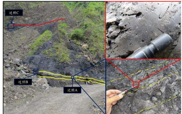
Figure 6. Field observation of faulted material in the study area.
