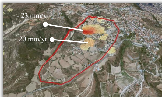
Figure 5: Vertical displacement of Area A with values up to -23mm/year using SBAS analysis
