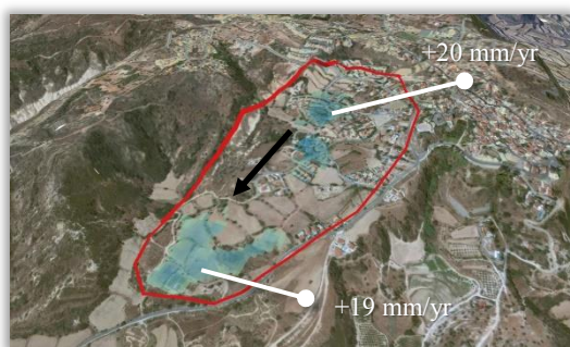
Figure 6: Horizontal displacement of Area A with values up to 20mm/year using SBAS analysis. Black arrow shows direction of movement
