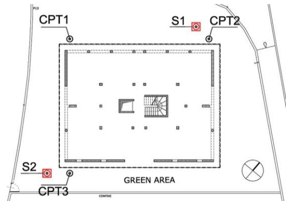
Figure 3. Plan of soil investigation, CPT and boreholes
