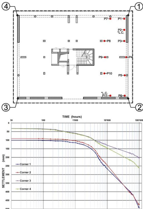
Figure 5. Settlement monitoring targets (C1-C4) and recorded values; plane above shows underpinning piles
