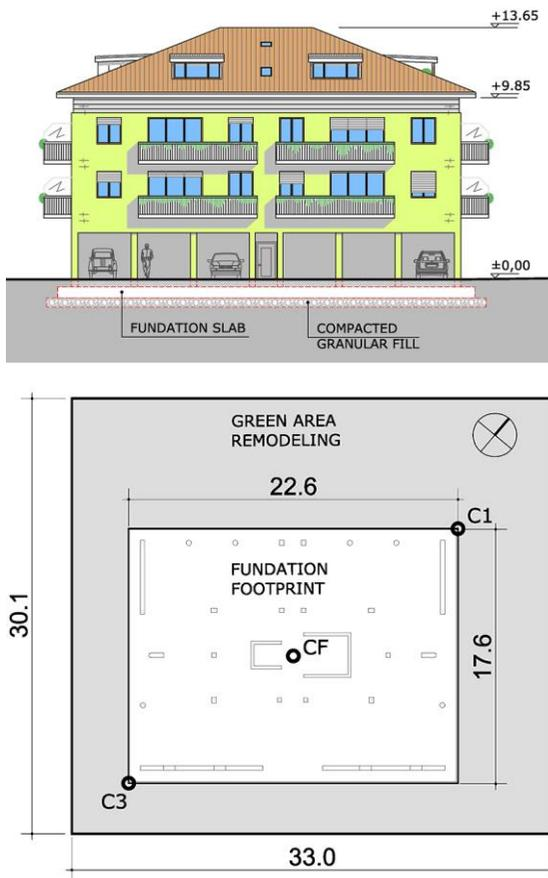
Figure 2. The longest façade, looking North, and the area of the building and the foundation slab (C1, C3, Cf: points where settlements have been calculated)
