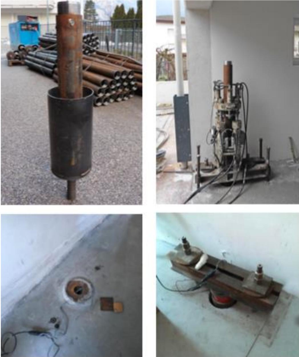
*Figure 6. Steel tube and base bucket (top left); pushing equipment with micropile (top right); load cell embedded into the slab foundation (bottom left); removable load cell between head of micropile and reaction frame (bottom right)*
