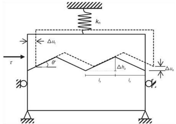
Figure 2. Conceptual model of dilatant joints (Heuze, 1979)
