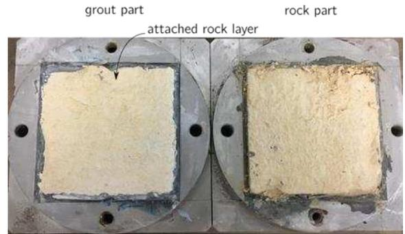
Figure 10. Shear surface of a soft limestone/gROUT interface tested under CNS
