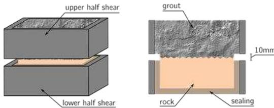
Figure 3. Schematic illustration of an interface sample
