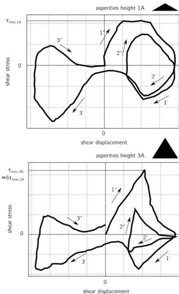
Figure 11. Shear surface of two calcarenite/grout interfaces of different roughness tested under CNS
