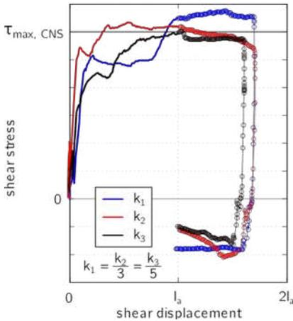
Figure 9. Shear resistance of a soft limestone/gROUT interface tested under CNS
