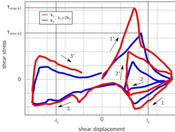
Figure 8. Shear resistance of two similar calcarenite/gROUT interfaces tested under different applied normal stiffness
