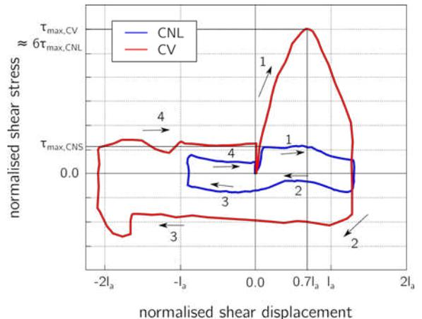
Figure 5. Shear resistance of a calcarenite/grout interface under CNL and CV
