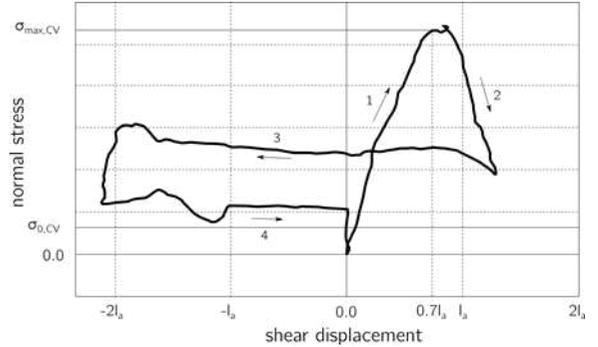
Figure 7. Evolution of the normal stress with shear displacement under CV
