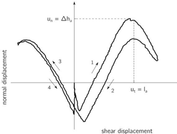
Figure 6. Dilation – contraction of a calcarenite/grout interface tested under CNL
