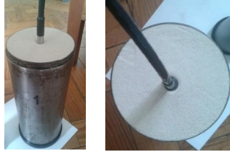
Figure 2- Thermal probe inserted in the sand sample during thermal conductivity measurements
