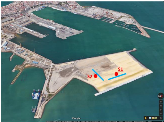
Figure 3. General view of the reclamation land and a sketch of the boreholes location and SASW spreads.
