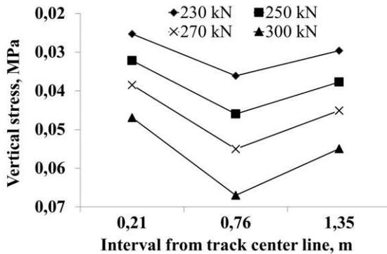
Figure 3. Vertical stress distribution at the level of 55 cm under sleeper
