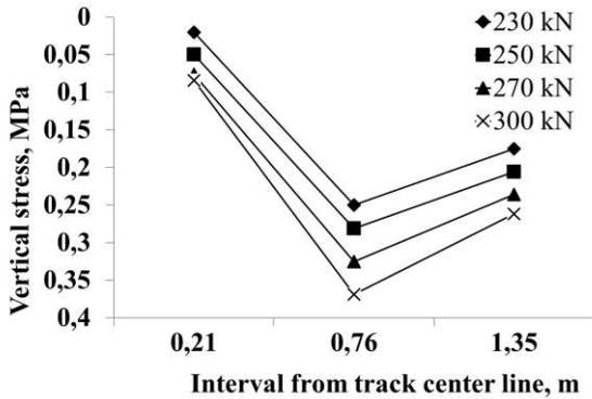
Figure 2. Vertical stress distribution at the level of 10 cm under sleeper
