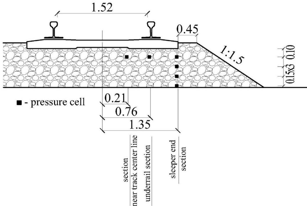
Figure 1. Sensor placement in ballast and subballast
