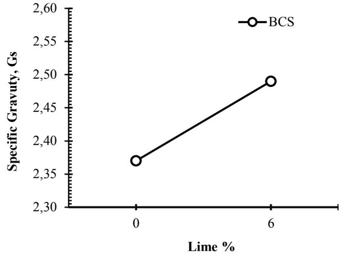
Figure 3. Variation of specific gravity of black cotton soil with addition of Lime.
