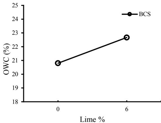
Figure 9. Variation of optimum water content of black cotton soil (BCS) with addition of lime.
