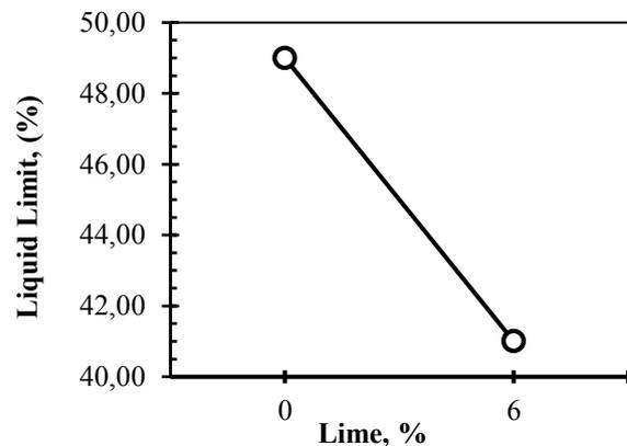
Figure 4. Variation of liquid limit of black cotton soil with addition of lime.
