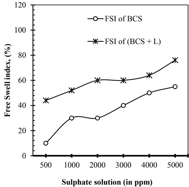
Figure 10. Free swell index of Black cotton soil with addition of lime in presence of sulphate contaminated water.
