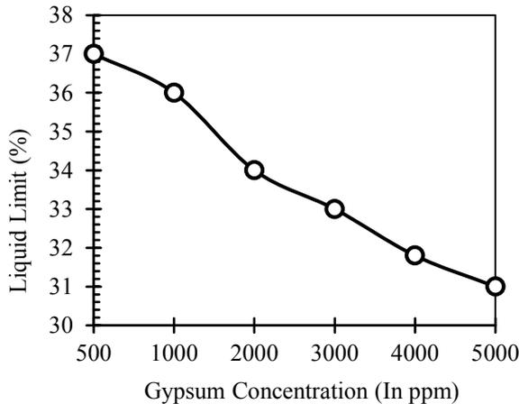
Figure 5. Variation of liquid limit of black cotton soil & lime in presence of sulphatic contamination
