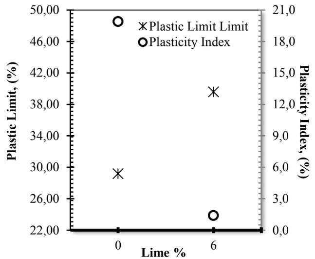
Figure 6. Variation of plastic limit and plasticity index of black cotton soil with addition of lime.
