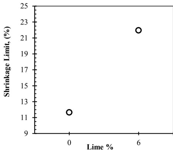
Figure 7. Variation of shrinkage limit of black cotton soil with addition of lime.
