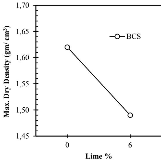
Figure 8. Variation of maximum dry density of black soil with addition of lime.
