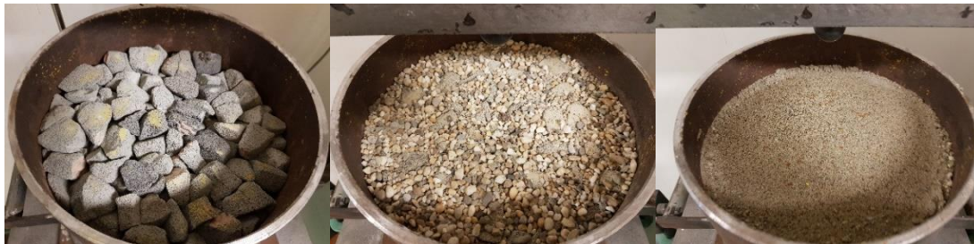
Figure 3. Foamglass aggregate laboratory sample preparation
