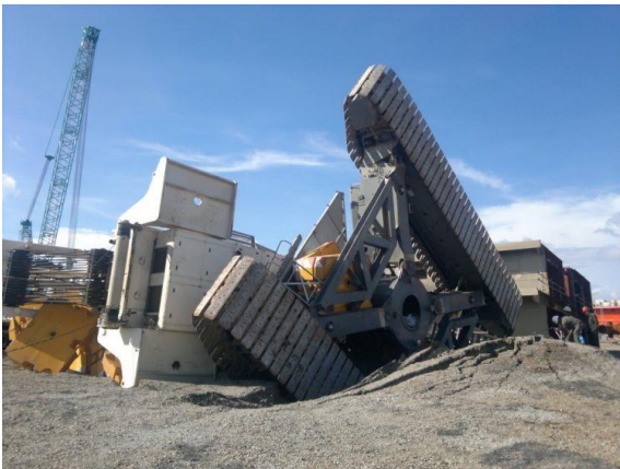
Figure 1: crawler crane accident caused by insufficient ground conditions ( www.simscrane.com )
