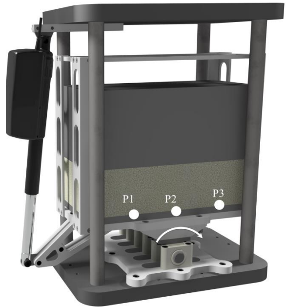
Figure 5. Schematic sketch of the newly developed static liquefaction triggering actuator for the geo-centrifuge at TU Delft
