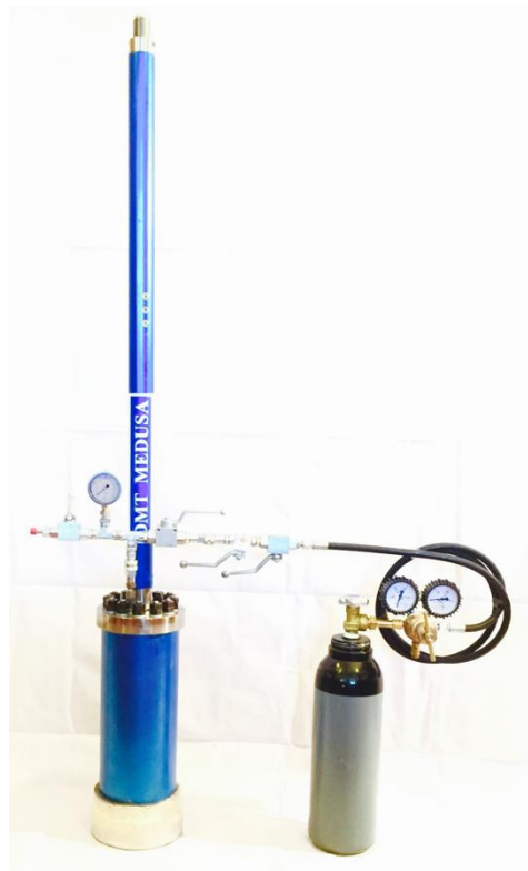
Figure 3. Calibration chamber used for preliminary tests on the Medusa DMT
