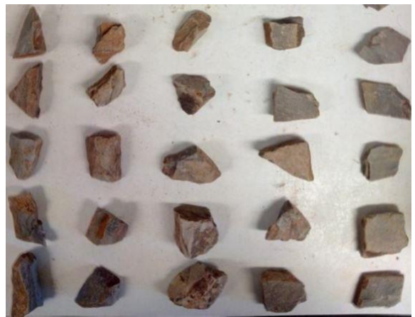
Figure 3. Gravel particles before testing by means of uniaxial tests
