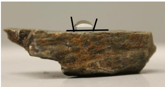
Figure 4. Measurement of the contact angles of a drop on a hydrophobic treated surface
