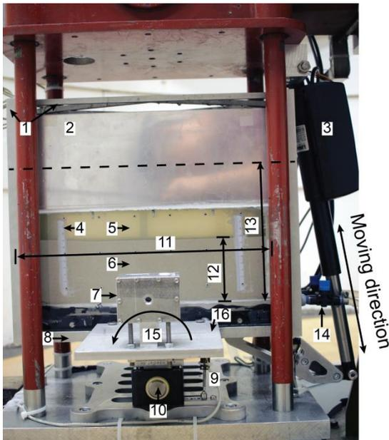
Figure 4. Front view of test setup after sample preparation (model scale): 1) outer frame; 2)
