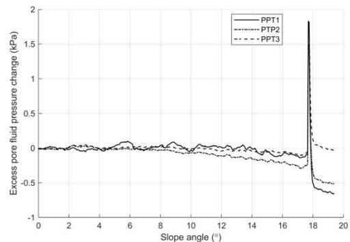
Figure 5. Changes in excess pore water pressure for Cent1
