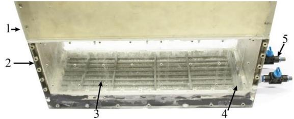
Figure 2. Fluidization system: 1) extension box; 2) strongbox; 3) parallel pipes; 4) transverse pipe; 5) valves
