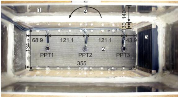
Figure 1. Top view of the newly developed strongbox with an integrated fluidization system at the base: 1) extension box; 2) fluidization filter; 3) PVC block; 4) tilting direction. (unit: mm, model scale)
