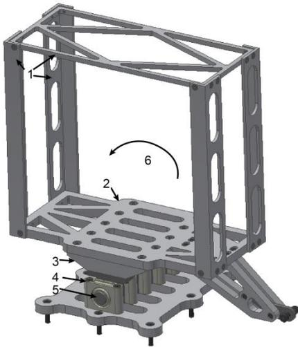
Figure 3. Schematic sketch of the newly developed tilting frame for triggering static liquefaction for the geo-centrifuge at TU Delft: 1) outer frame; 2) base plate; 3) bearing blocks; 4) shaft blocks; 5) rotating axis; 6) rotating direction
