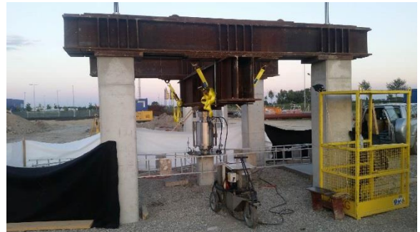
Figure 8. Static pile load test setup
