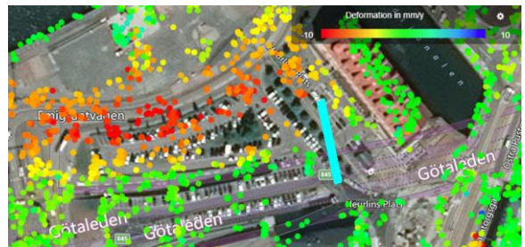
Figure 5. Data from satellite monitoring showing rate of on-going settlements at ground surface level (green=0 mm/year to red \geq 10 mm/year) with section 1/430 highlighted in blue.
