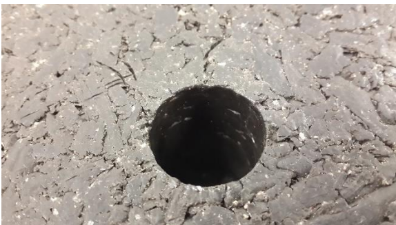
Figure 4. Augered pile hole (diameter 20 mm)
