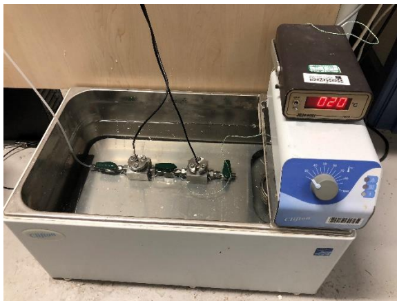
Figure 4. Tensiometers submerged in the temperature-controlled water bath
