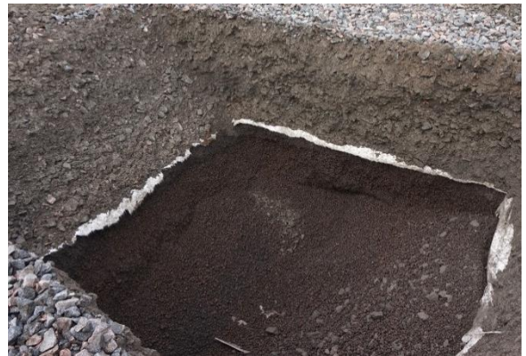
Figure 9 The excavation of non-compacted LWA structure with natural water content (Photo: T. Dettenborn 08/2017)
