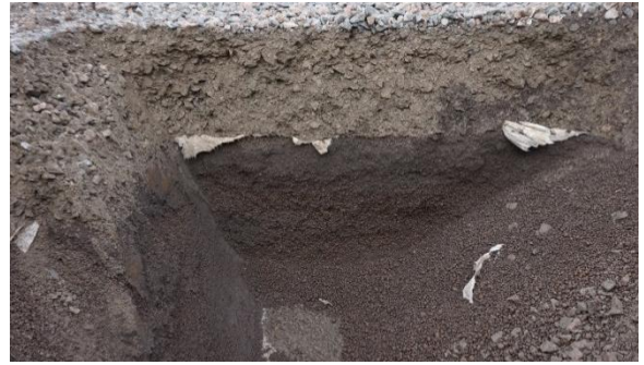
Figure 8 The excavation of compacted LWA structure with natural water content (Photo: T. Dettenborn 08/2017)
