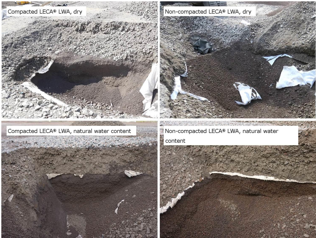
Figure 10 Effect of the compaction and the water content in LWA structures. Top left: compacted LWA in dry conditions. Top right: non-compacted LWA in dry conditions. Bottom left: compacted LWA in natural water content. Bottom right: non-compacted LWA in natural water content. (Photo: S. Frimodig and T. Dettenborn 08/2017)
