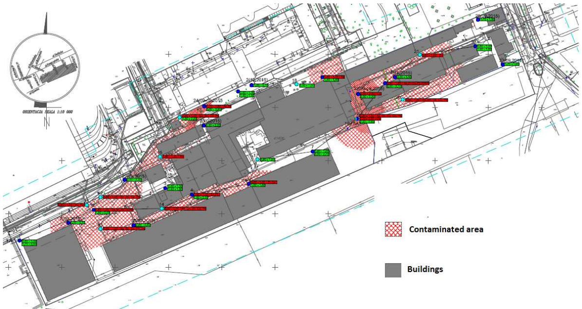
Figure 9. Map of soil quality at depth of 0.25 m below ground level or lower, Objazdowa Street
