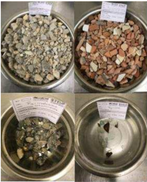
Figure 2. Example of the constituents of the recycled aggregate after hand sorting
