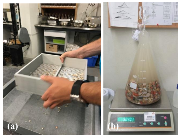
Figure 3. Characterization of the recycled aggregate: a) determination of flakiness index; b) determination of particle density and water absorption
