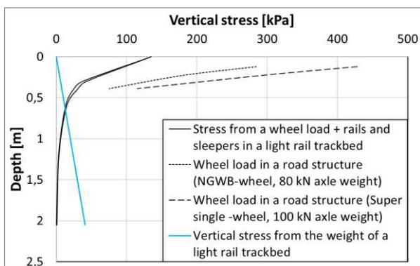
Figure 2. Comparison of vertical stresses in a light rail trackbed and a road structure (Linden 2018)
