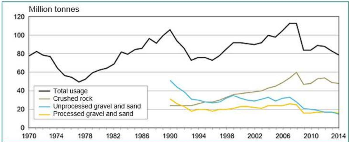
Figure 1. Estimated natural rock aggregate usage in Finland in 1970–2014 (adapted from Geological Survey of Finland 2017)
