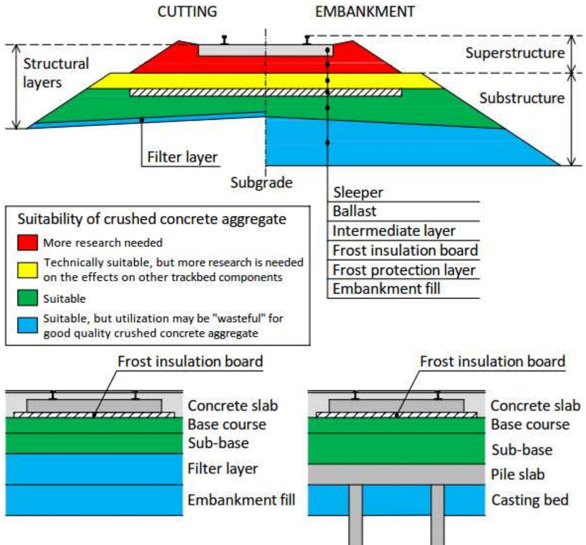
Figure 3. Components of different types of light rail tracks and the suitability of CCA use in the various layers (Linden 2018)
