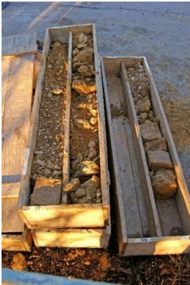
Figure 2. Drill core samples
