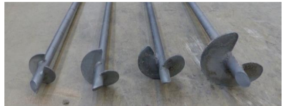
Figure 3. Model anchors S4 to S7 (from left to right)
